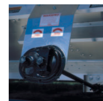
Two Speed Door Openers; Two speed operators are optional on the Low-Torque door system for applications where high density products are being hauled.
