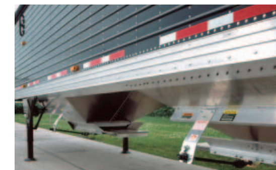
Two-piece Formed Ag Tub Option; By utilizing two aluminum panels per tub rather than four, all welds and rivets in the corners that could impede the flow of product have been eliminated. This design is standard on Timpte's high ground clearance models.
