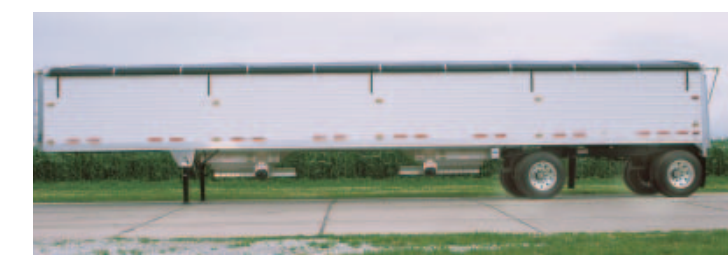
Spread Axle Models; Available in lengths of 48' to 50'. Axle spacings available from 10'-2" to 10'-8". Air-ride suspensions are standard on all Spread Axle trailers.
