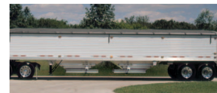
Standard Split Tub Hoppers; These hoppers are standard on all models from 40' to 50' in length. Available on both 96" and 102" wide trailers. This tub offers 17" of ground clearance and full access to the apex of the trailer.
