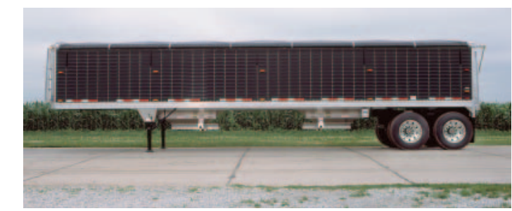
Optional Formed Ag Hoppers; This option is available on all models from 40' to 50' in length. Available on both 96" and 102" wide trailers. Designed with 25" of ground clearance for applications where a swing under unloading auger is needed.
