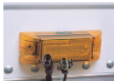
Electrical; All weather-pack automotive style connections, sealed to prevent corrosion.
