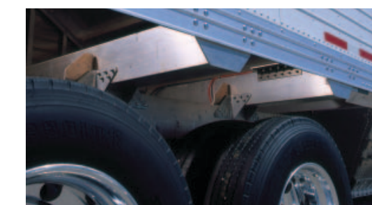
Optional Aluminum Sub-Frame; For maximum weight reduction Timpte offers this option on most trailer models.
