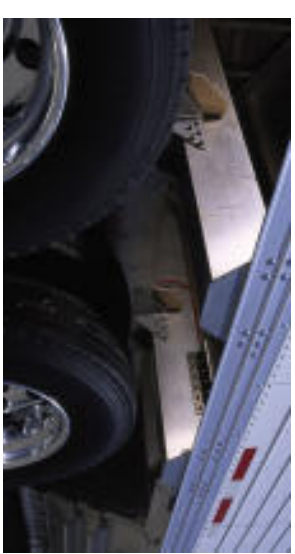
Optional Aluminum Sub-Frame. For maximum weight reduction Timpte offers this option on most trailer models.
