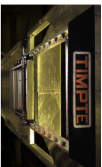
Low-Torque Trap Doors. Standard on all trailer models. A 50% reduction in the effort required to open these Low-Torque doors is realized by having the door ride on sealed ball bearings.
