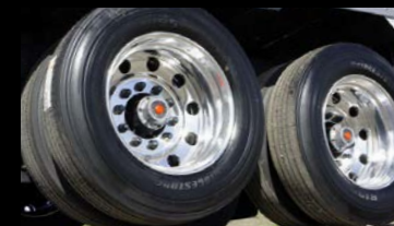
For less weight and more payload many customers choose all aluminum wheels.
