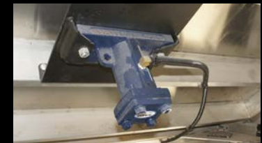
Air operated vibrators improve product clean out, and can be mounted on all hopper tubs.
