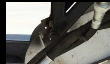
Removal of the upper belt assemble consist of removing a single pin at the transition and unhooking the hydraulics.
