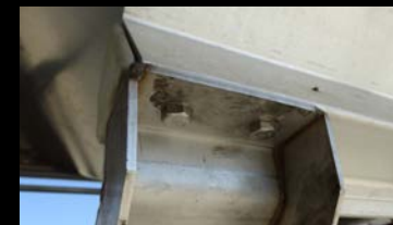
Removal of 12 bolts makes it easy to disconnect the lower belt assemble.
