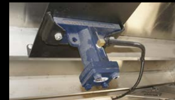
Air operated vibrators improve product clean out, and can be mounted on all hopper tubs.
