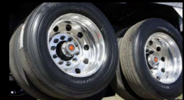
For less weight and more payload many customers choose all aluminum wheels.
