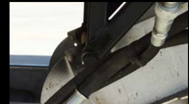
Removal of the upper belt assemble consist of removing a single pin at the transition and unhooking the hydraulics.
