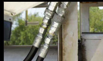
Timpte utilizes quick couplers for removal of all hydraulic hoses.
