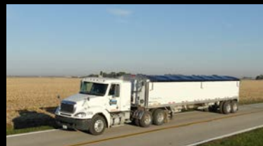
Belt system can be removed in about one hour and the trailer can be used as a standard conventional grain hopper.
