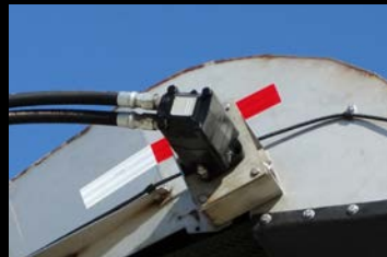
The upper and lower assembly units utilize hi-performance Parker hydraulic motors.
