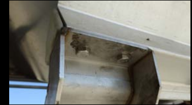
Removal of 12 bolts makes it easy to disconnect the lower belt assemble.
